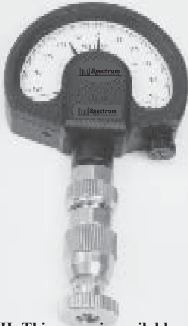
Type H: This gauge is available with a resolution of 0.005mm, or 0.0001 inches.
