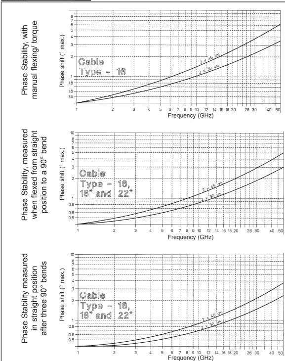
Diagrams: Three different criteria were determined to demonstrate the max. phase shift of the cables at ambient temperature. Tests were performed on pairs of cables, so that the total lengths of the assemblies under test were always 60 cm and 90 cm respectively.
