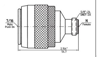
Dimensions shown are inches over millimeters. Standard units have stainless steel finish (last two digits of the P/N are -02). Interfaces are per MIL-C 39012, MIL-C-87104/2, MIL-C-3643, MIL-STD-348, IEC-169-7, IEC-457-2, DIN 47 223, DIN 47 226, DIN 47 298, where applicable. For details please refer to the beginning of this section.
