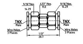
Dimensions shown are inches over millimeters. Standard units have stainless steel finish (last two digits of the P/N are -02). Interfaces are per MIL-C 39012, MIL-C-87104/2, MIL-C-3643, MIL-STD-348, IEC-169-7, IEC-457-2, DIN 47 223, DIN 47 226, DIN 47 298, where applicable. For details please refer to the beginning of this section.
