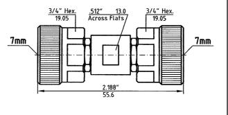
Dimensions shown are inches over millimeters. Standard units have stainless steel finish (last two digits of the P/N are -02). Interfaces are per MIL-C 39012, MIL-C-87104/2, MIL-C-3643, MIL-STD-348, IEC-169-7, IEC-457-2, DIN 47 223, DIN 47 226, DIN 47 298, where applicable. For details please refer
