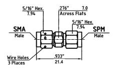
Dimensions shown are inches over millimeters. Standard units have stainless steel finish (last two digits of the P/N are -02). Interfaces are per MIL-C 39012, MIL-C-87104/2, MIL-C-3643, MIL-STD-348, IEC-169-7, IEC-457-2, DIN 47 223, DIN 47 226, DIN 47 298, where applicable. For details please refer to the beginning of this section.
