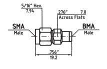
Dimensions shown are inches over millimeters. Standard units have stainless steel finish (last two digits of the P/N are -02). Interfaces are per MIL-C 39012, MIL-C-87104/2, MIL-C-3643, MIL-STD-348, IEC-169-7, IEC-457-2, DIN 47 223, DIN 47 226, DIN 47 298, where applicable. For details please refer to the beginning of this section.
